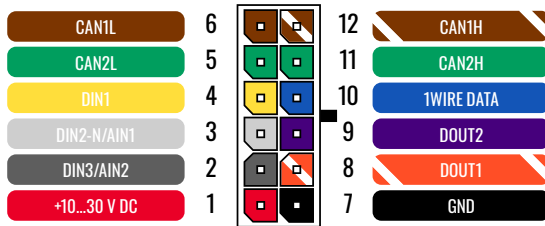
FMB150-QJIB0 pinout
