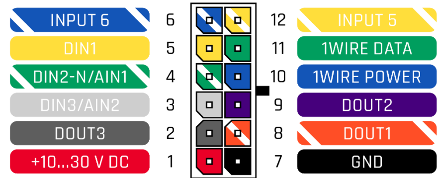
Figure 2 FMC130 2x6 socket pinout
